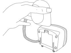
2. Insert the batteries the correct way up. The orientation is marked in the battery compartment.
