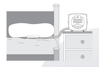
2. In the event of a fire, the pillow pad will vibrate and the unit will flash. The word 'fire' will also be present on the display.
