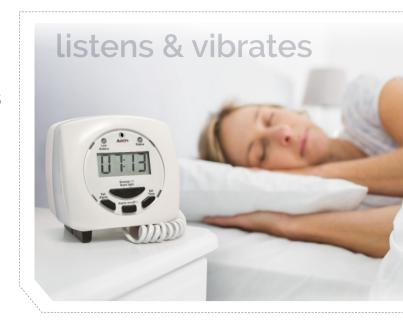
The Agrippa pillow alarm is a battery powered, wire-free unit with a pad attachment that simply goes under a pillow. It uses digital wire-free technology that listens for the unique sound of a specific fire alarm.
