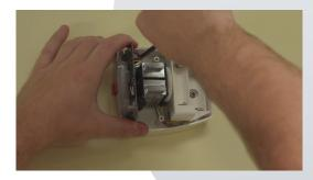
Fit the supplied batteries (2 x "C" cells). Note, the correct orientation is marked in the battery compartment. The motor will turn for around five seconds.
